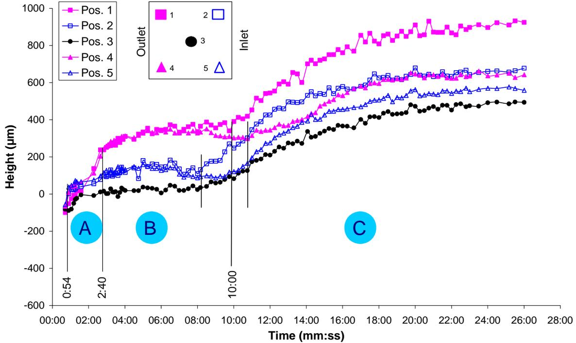
Fig. 4 Thickness change as a function of time measured at 5 locations over the plate during infusion.
