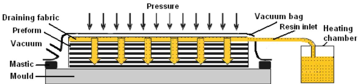
Fig. 1 Principle of LRI processes [1]
