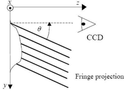
Fig.2 Basic principle of fringe projection.
