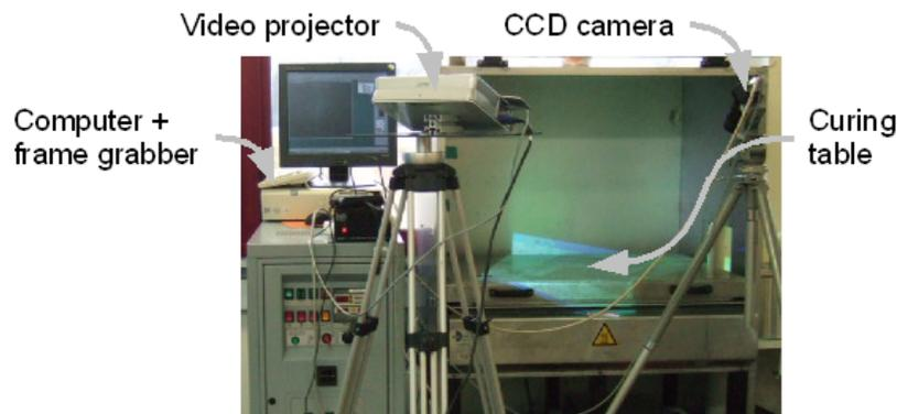
Fig.3 Experimental testing device
