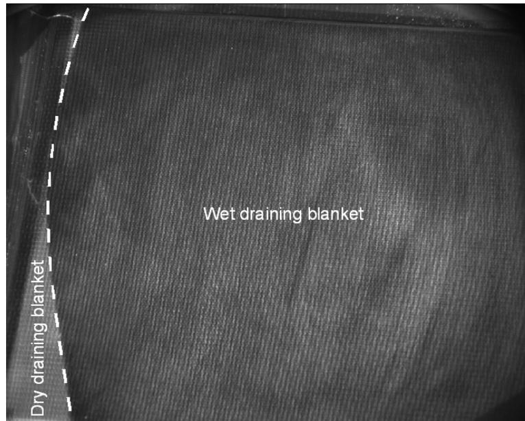
Fig.5 Resin propagation in the draining fabric.
